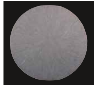
Sectional view of crack-free bloom format
