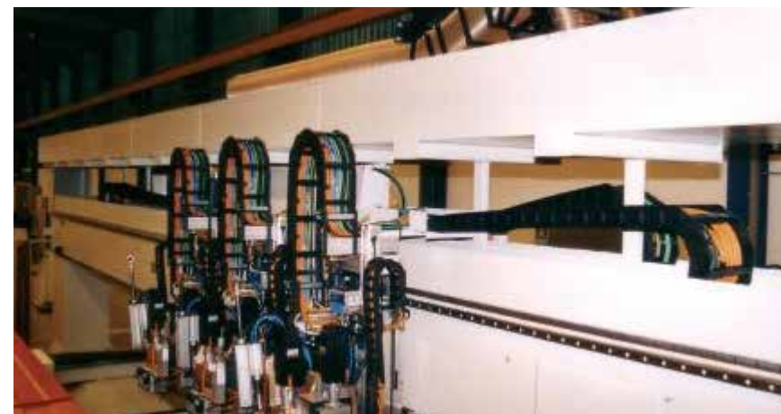
Woodworking machines with e-chains® and chainflex® cables
