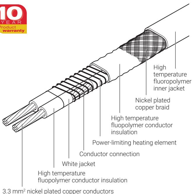
nVent RAYCHEM VPL is a family of power limiting heating cables designed for pipe and equipment heat-tracing in industrial applications.
