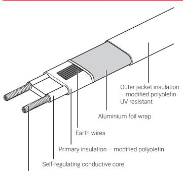
The nVent RAYCHEM BSA self-regulating heating cable is designed for industrial pipe freeze protection without steam cleaning and moderate process temperature requirements. It can be used for indoor and outdoor installation in ordinary (non-hazardous) area applications.
