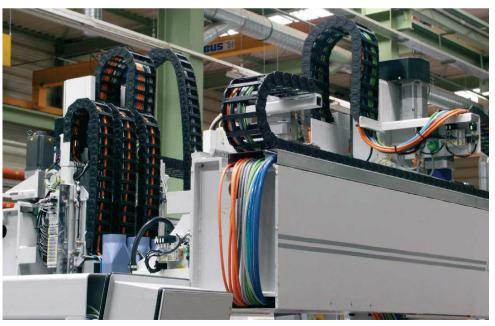
Many e-chains® are used in this customised CNC-machine for the woodworking industry
