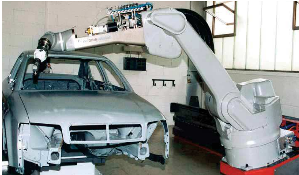
Paint spraying robot with system E4 e-chains® in ESD version. High rates of acceleration of up to 6m/s 2 and high braking rates for a robot weight of approx. one ton
