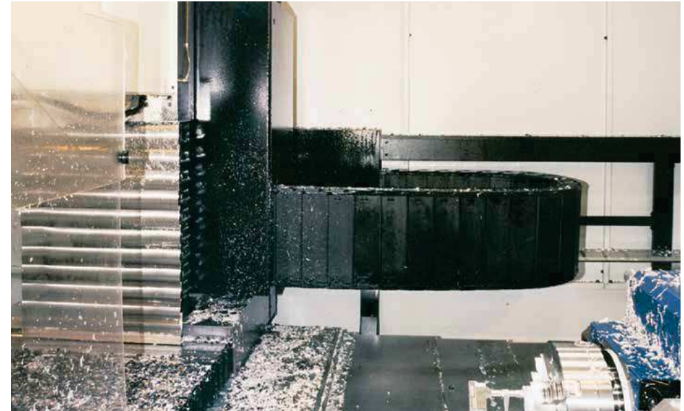
Side-mounted E4/light e-tubes - machine tool fitted with a swarf-repellent e-tube from the E4 modular system
