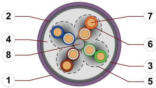
1. Outer jacket: Pressure extruded, halogen-free TPE mixture
