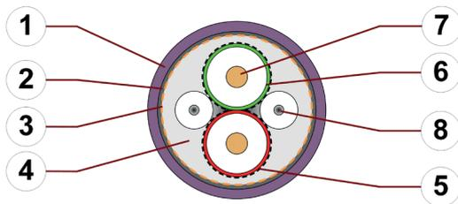
1. Outer jacket: Pressure extruded, halogen-free TPE mixture
