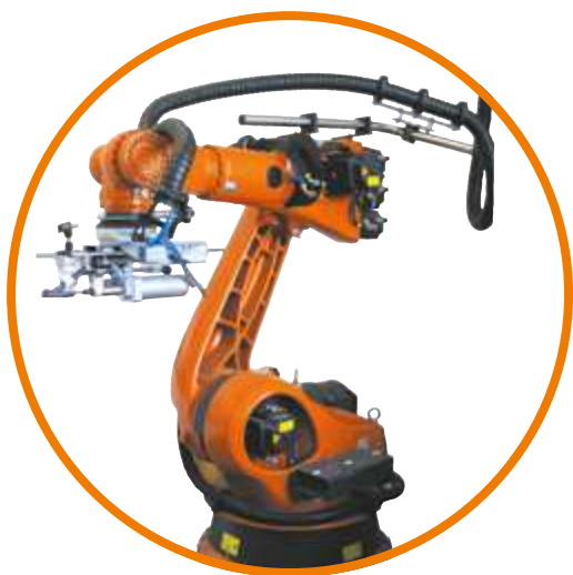
Fibre rod module on a universal assembly kit (aluminium tube).
