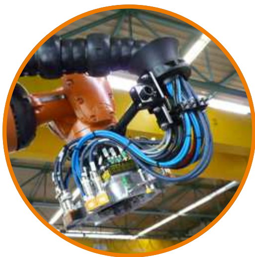
Radius support provides additional stability when connecting e-chain® and mounting bracket
