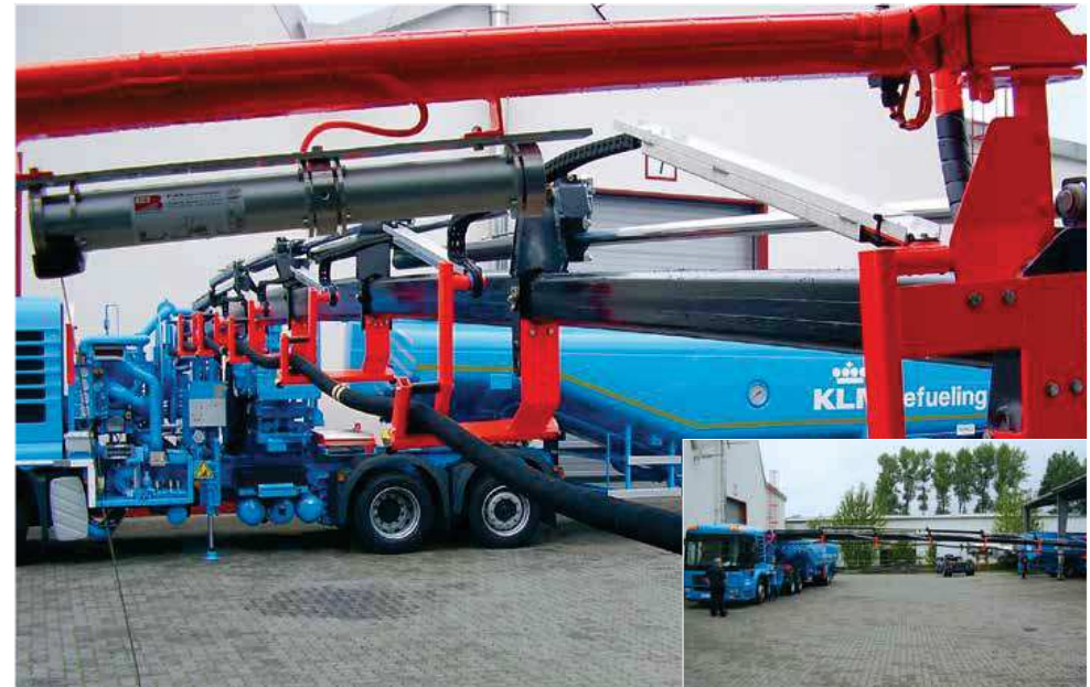
E2/000 series 1400 in aircraft refuelling truck - telescopic crane with six sections
